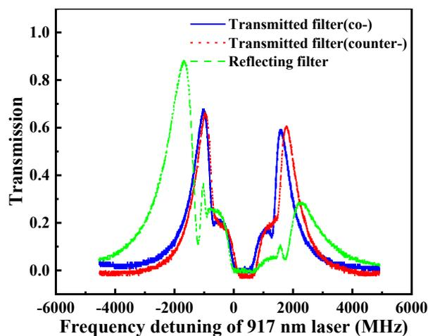
Fig. 8 Reflection-type ES-FADOF and traditional transmitted ES-FADOF with co-propagating and counter-propagating experimental configurations
